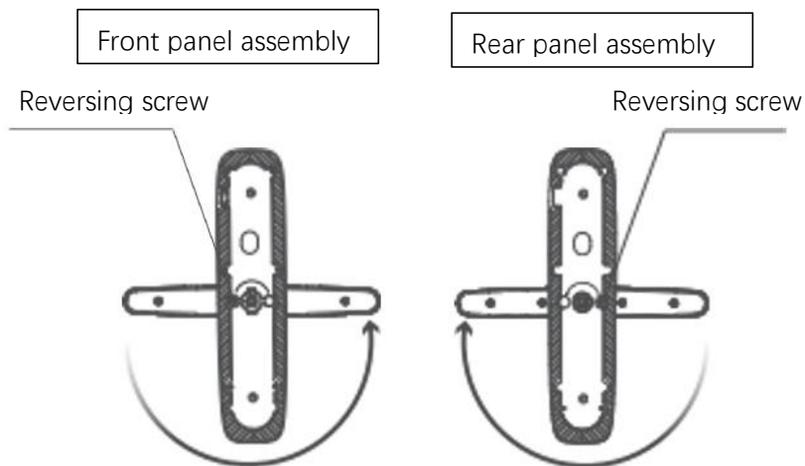
Use a screwdriver to remove the reversing screw, turn the handle 180 degrees counterclockwise to reverse, and tighten the reversing screw on the other side after reversing.
